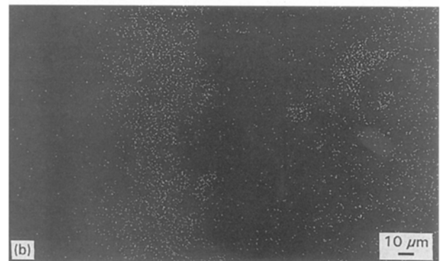
Figure 18 (a) A scanning electron micrograph of the solid Ni/solid Ag-28 wt % Cu diffusion couple annealed at 700 °C for 8 weeks. (b) Cu-elemental X-ray mapping of the solid Ni/solid Ag-28 wt % Cu diffusion couple annealed at 700 °C for 8 weeks.
